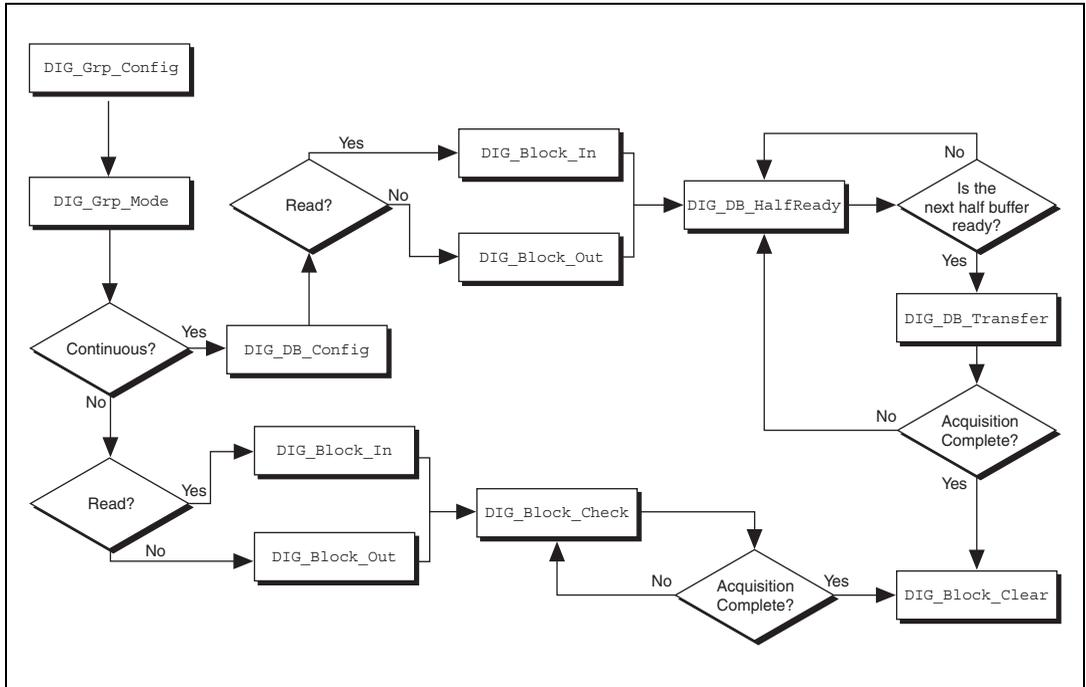
Figure 2-4. Programming Buffered Handshaking I/O in NI-DAQ
