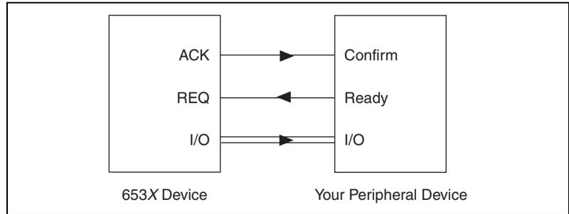
**Figure 2-3.** Connecting Signals
