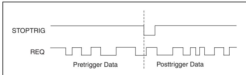
Figure 2-17. Stopping Data Transfer Using a Trigger
