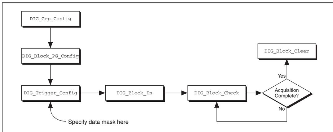
**Figure 2-21.** Programming Change Detection (Single Buffer) in NI-DAQ
