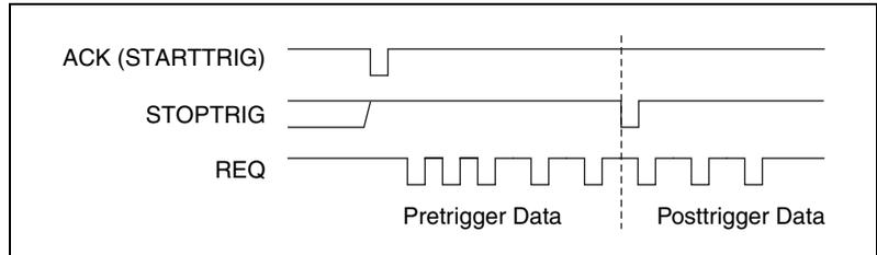
**Figure 2-18.** Using a Start and Stop Trigger
