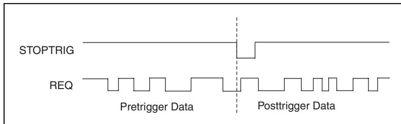
**Figure 2-9.** Stopping Data Transfer Using a Trigger
