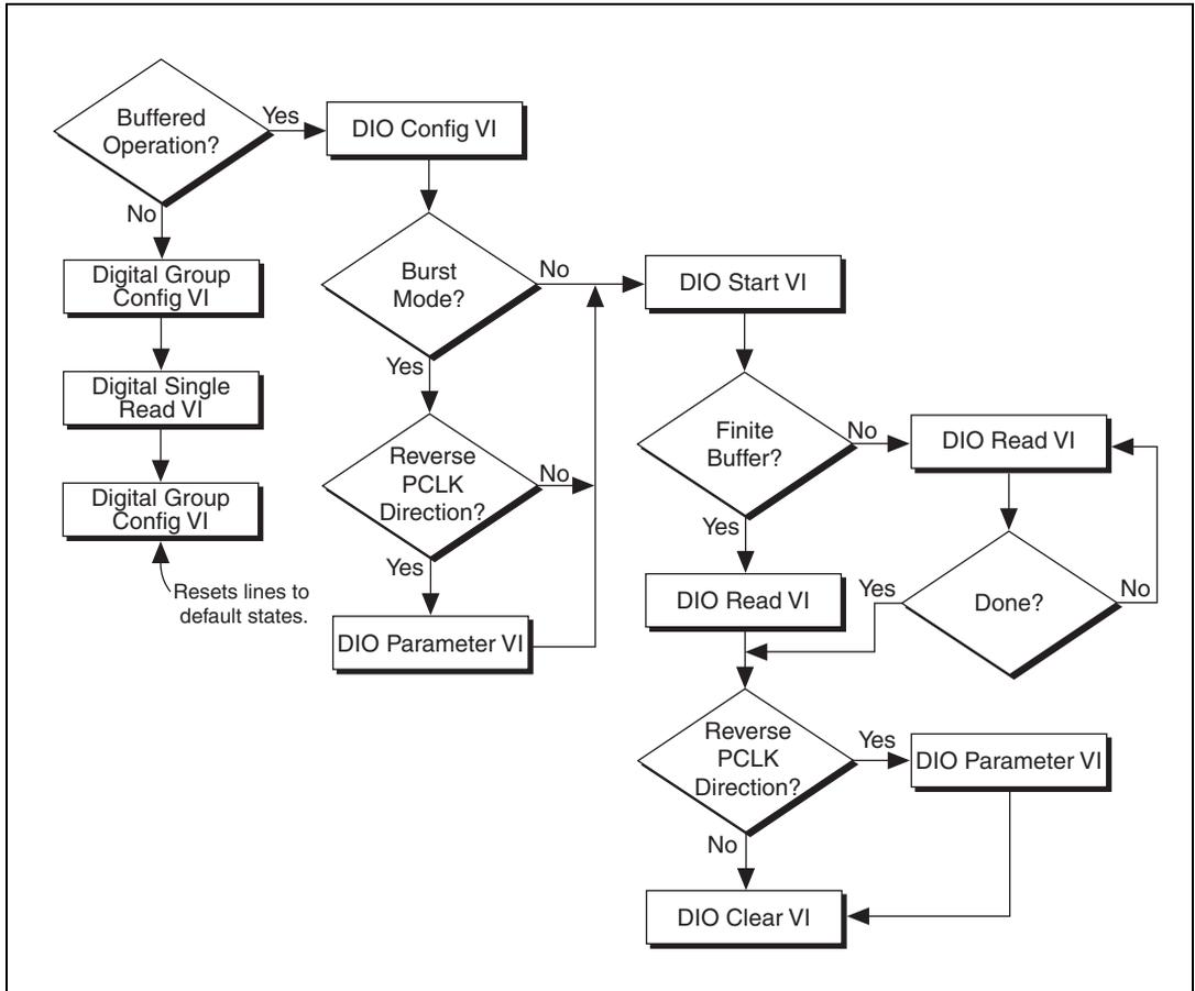
**Figure 2-6.** Programming Handshaking Input in LabVIEW/LabVIEW RT
