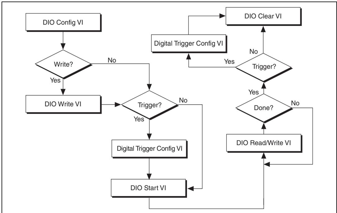
**Figure 2-14.** Programming Pattern I/O in LabVIEW/LabVIEW RT
