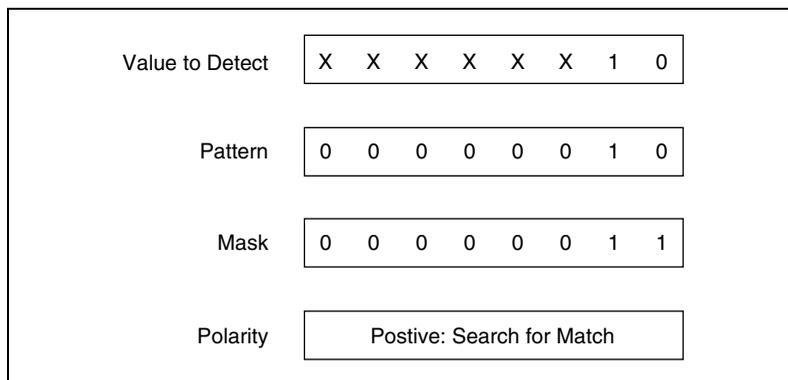
**Figure 2-19.** Pattern-Detection Trigger Example
