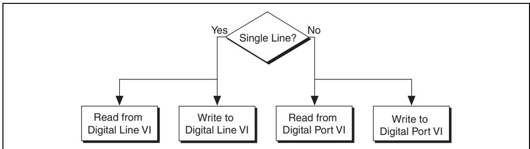
Figure 2-2. Programming Unstrobed I/O in LabVIEW/LabVIEW RT
