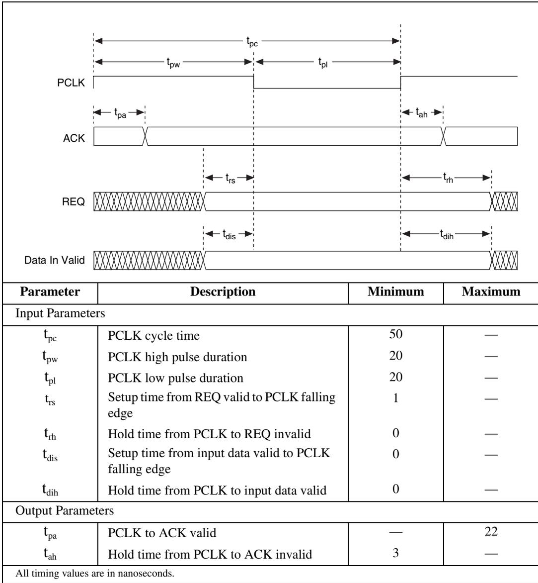
Figure 3-7. Burst Input Timing Diagram (PCLK Reversed)
