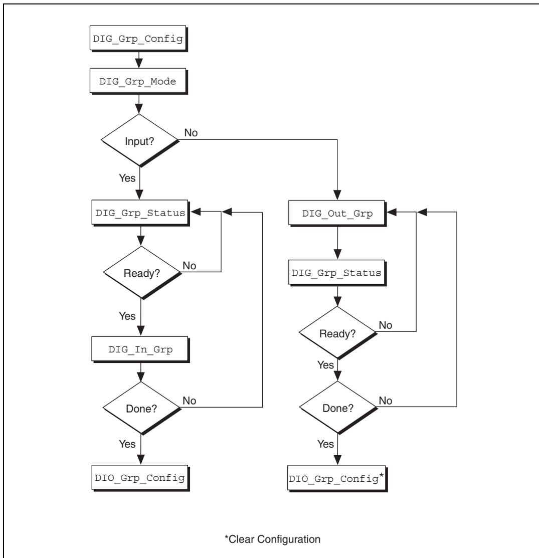
**Figure 2-5.** Programming Unbuffered Handshaking I/O in NI-DAQ
