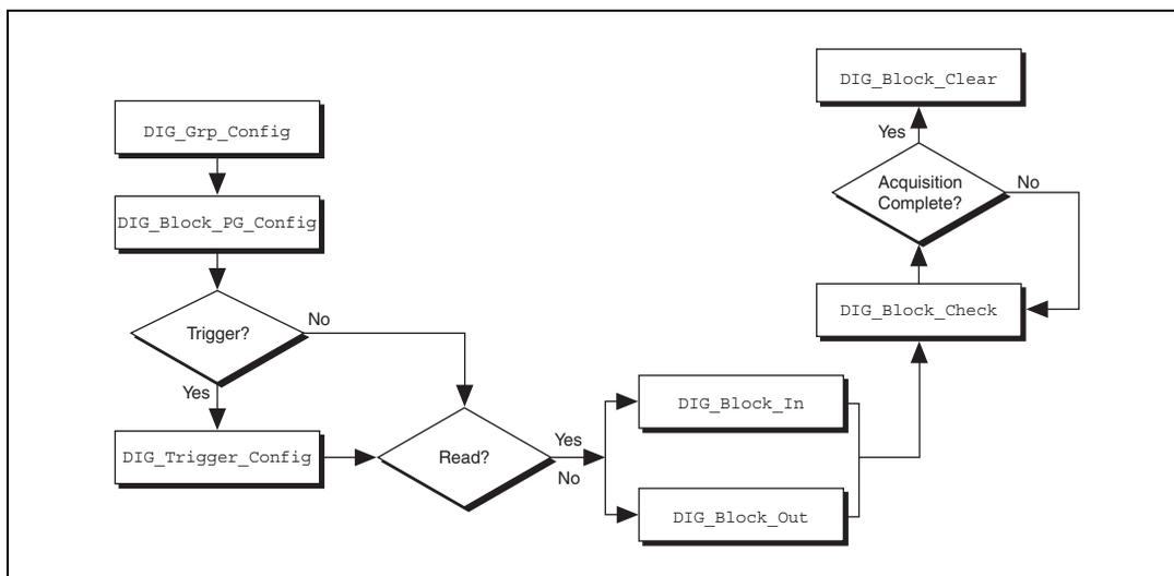
**Figure 2-12.** Programming Pattern I/O (Single Buffer) in NI-DAQ
