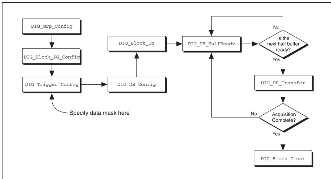
**Figure 2-20.** Programming Change Detection (Continuous) in NI-DAQ
