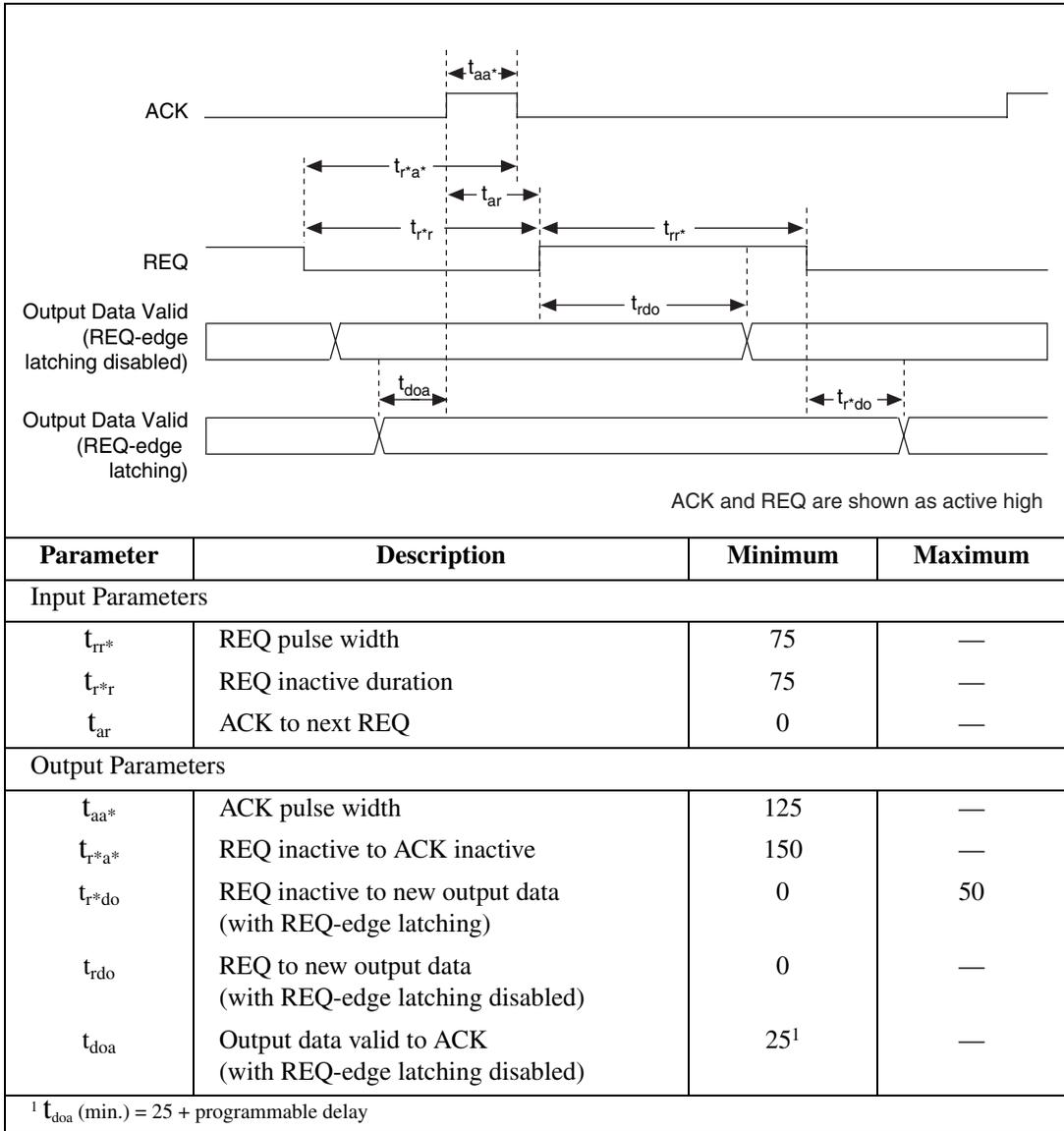
**Figure 3-31.** Leading Edge Output Timing Diagram
