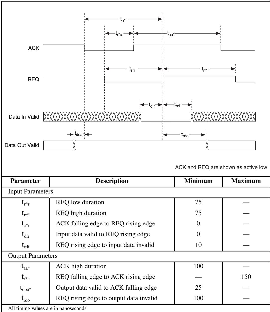
Figure 3-13. 8255 Emulation Output Timing Diagram
