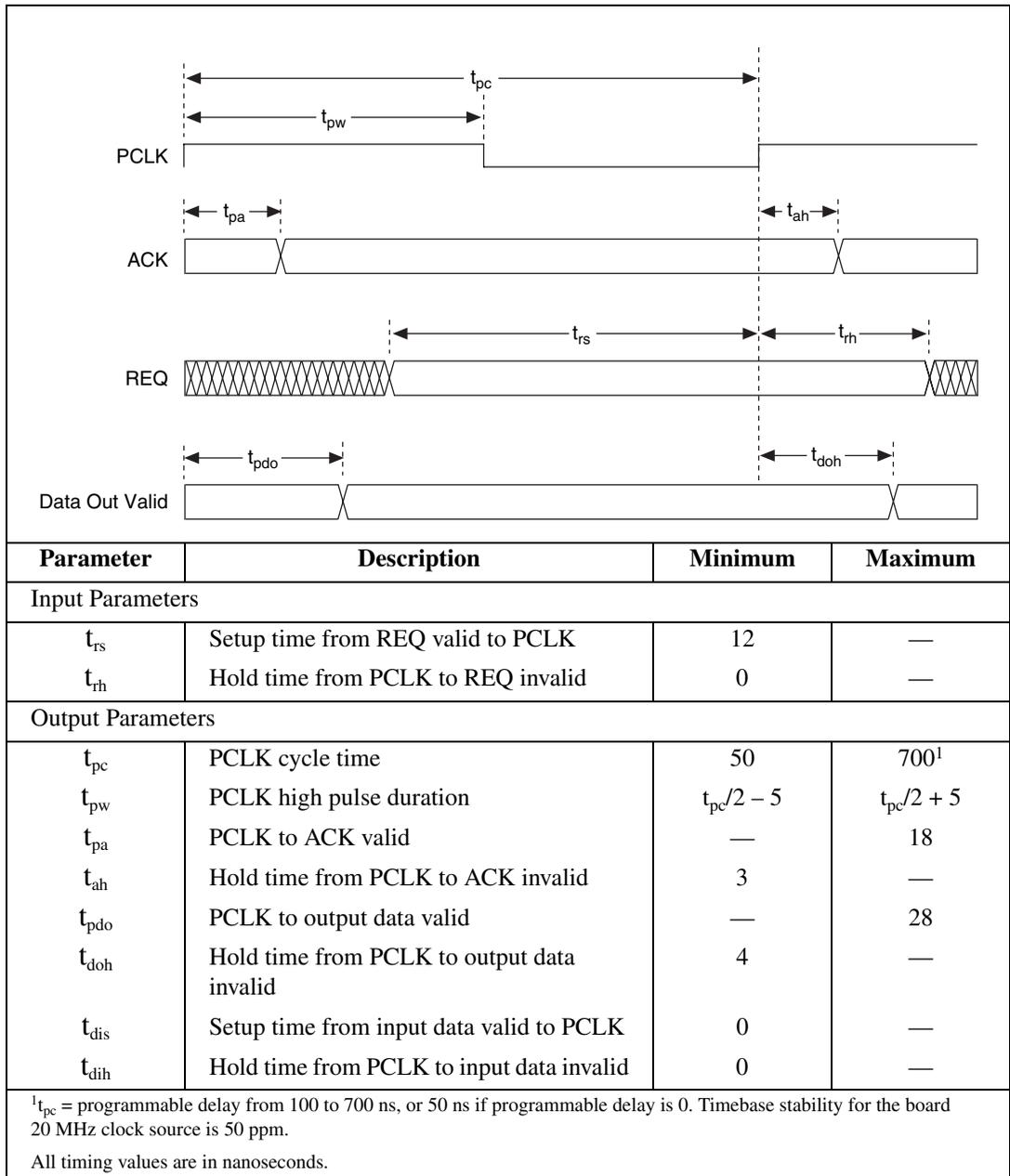
Figure 3-8. Burst Output Timing Diagram (PCLK Reversed)
