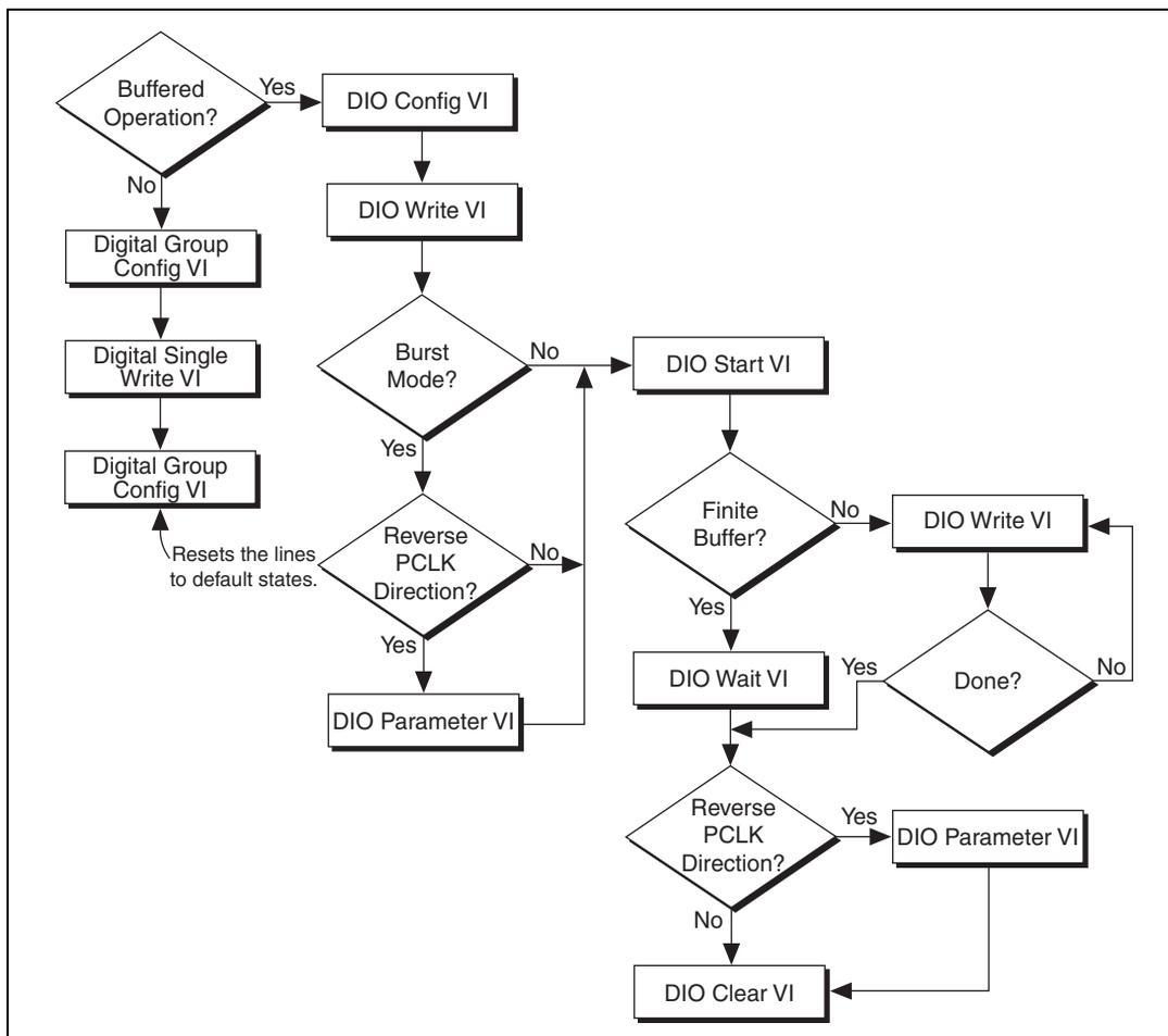
**Figure 2-7.** Programming Handshaking Output in LabVIEW/LabVIEW RT
