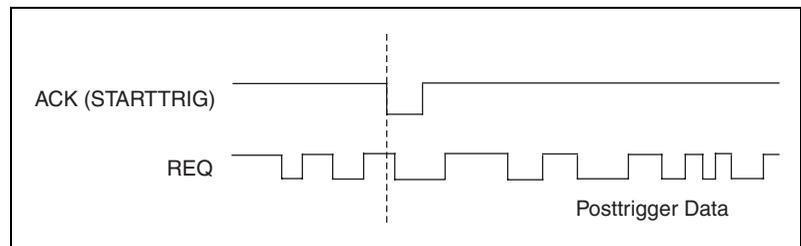
**Figure 2-8.** Starting Data Transfer Using a Trigger
