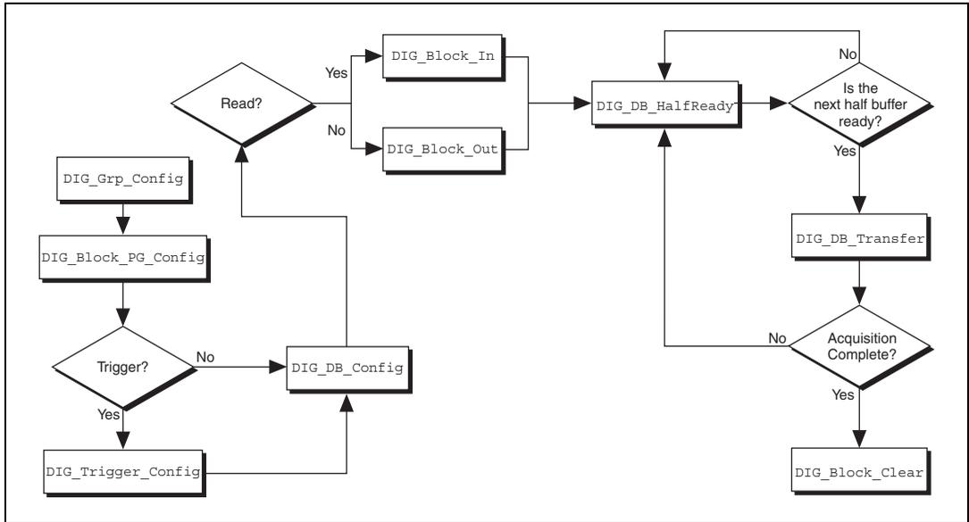
**Figure 2-13.** Programming Pattern I/O (Continuous) in NI-DAQ
