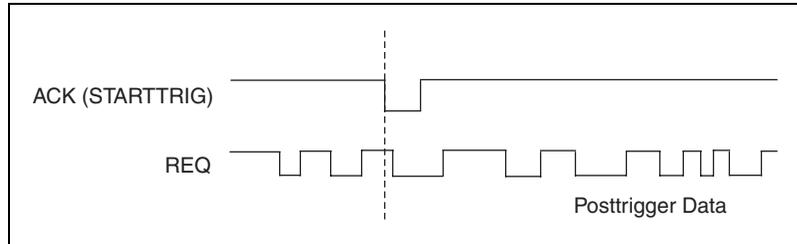
Figure 2-16. Starting Data Transfer Using a Trigger
