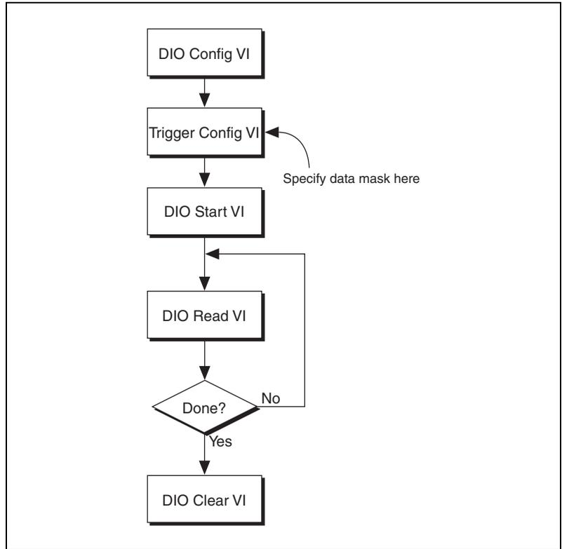
**Figure 2-22.** Programming Change Detection for LabVIEW/LabVIEW RT
