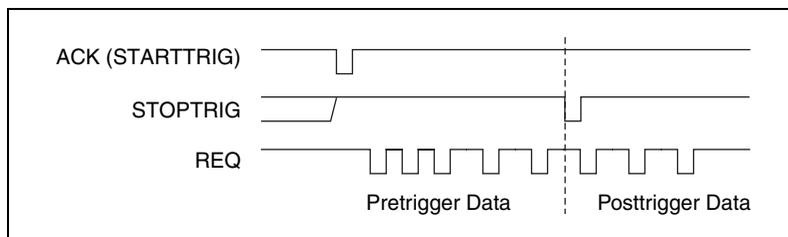
**Figure 2-10.** Using a Start and Stop Trigger
